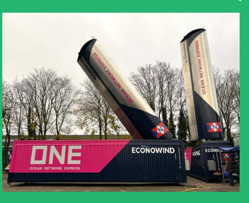
ONE announce the launch of a new trial aimed at unlocking the potential of wind propulsion as a sustainable solution for the maritime industry. We're installing two containerized wind assist devices, known as VentoFoil containers, on the MV Kalamazoo.
